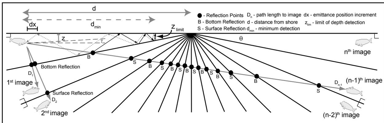
**Figure 4:** Geometrical ray tracing of a wedge shaped beach. To determine the total distance travelled by the ray and the number of reflections it undergoes it is best to 'unfold' the geometrical cross section of the beach into n - virtual isosceles triangles. The number n depends on the angle of the gently sloping beach.
